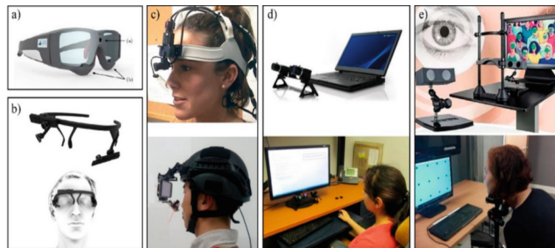
Fig. 1. Example of the different types of eye tracking devices: (a) eye tracking glasses; (b) headband; (c) helmet-mounted; (d) remote or table; (e) tower-mounted [38].
