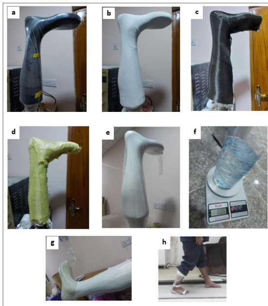
Fig. 3. Preparing the Negative Gypsum Pattern
